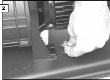
2 Attach the pump to the pedestal with the enclosed bolts (+nuts and washers).
